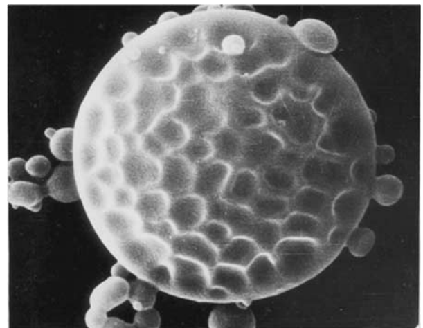
Figure 14 SEM image of a golf ball shaped PMMA particle.
